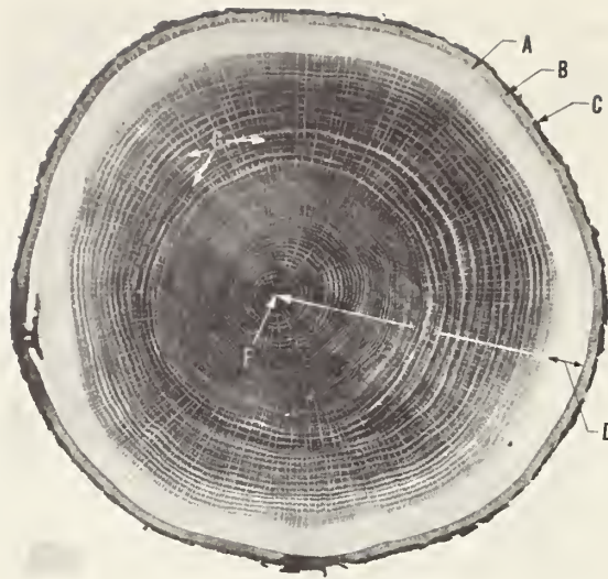
Figure 1. --Cross section of an oak tree. A is the microscopic cambium or growth layer; B, inner bark; C, outer bark; D, sapwood; E, heartwood; F, pith; and G, wood rays.
